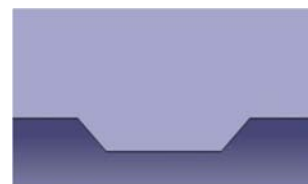
(c) Zoomed view of modified rectangular corner cavity L/D=6 .
