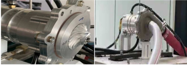
Figure 6. Prototype compressor and motor.
